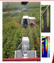
FTS for vertical sounding of the atmosphere for 3D maps of composition (H<sub>2</sub>O, CO<sub>2</sub>, O<sub>3</sub>, N<sub>2</sub>O, CH<sub>4</sub>, etc.) and temperature
